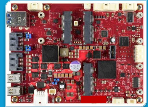
High density PCBA 1200+ placements on top side 800+ placements bottom side SMT, TH and Mechanical
