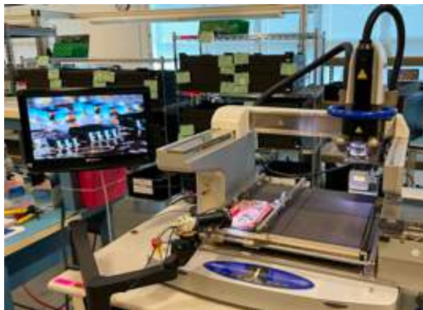
Onyx 29 Semi-Automated Rework System with integrated force measurement and vision system. For PCBAs up to 500 x 500mm.
